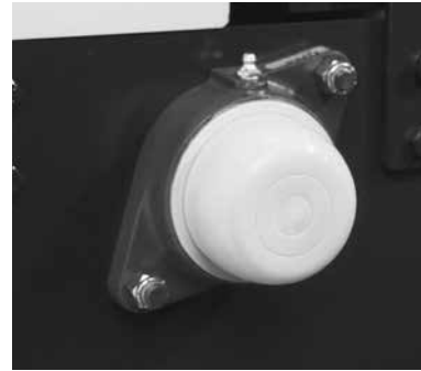
Fig. 29. Safety end caps protect against rotating stub shafts.
