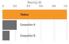
Comparison testing with 575 Series bearings from OE bearing manufacturers A and B. Information derived from Timken Accelerated Life Testing, using significant statistical samplings of bearings in a controlled test environment.
