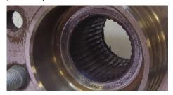
**POOR PERFORMANCE**: Bearing cone can turn on the hub barrel, which changes the bearing setting – promoting vibration, excessive noise and premature wear.
