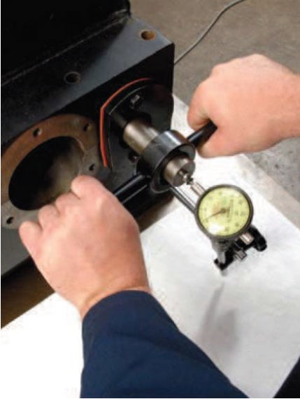
Figure 5: Example of Push / Pull Method on Industrial Gearbox Application.
