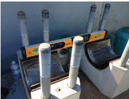
Figure 14: Torque Arm Alignment Measurement
