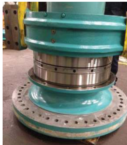
Figure 11: Pillow-Block Install over TDI
