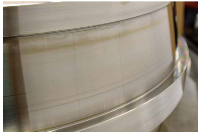
Figure 20: Bearing cone raceway
