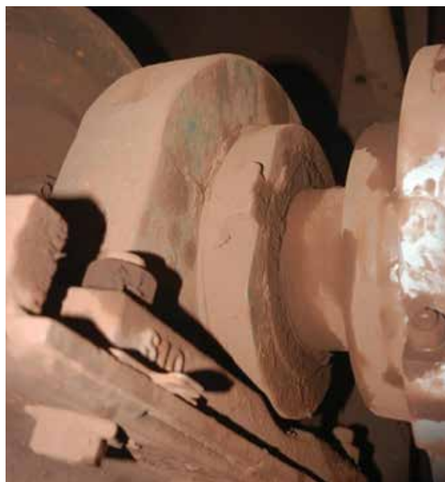
Fig. 20. Timken Mounted Split Cylindrical Roller Bearing is shown here in a steel industry application.
