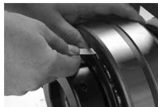
Measure RIC before installation.
