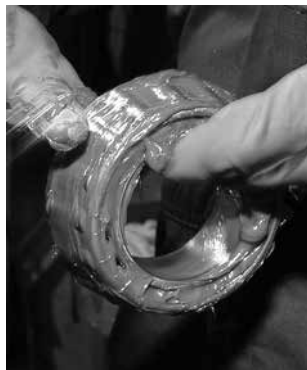
Fig. 149. Grease can easily be packed by hand.
