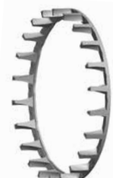
Fig. 46. Split, machined-brass, land-riding, finger-type cage.
