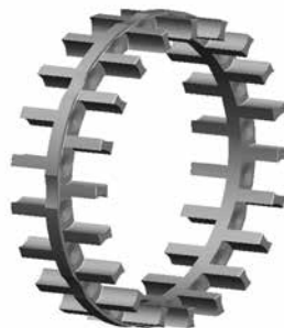
Fig. 49. One-piece finger-type cage.
