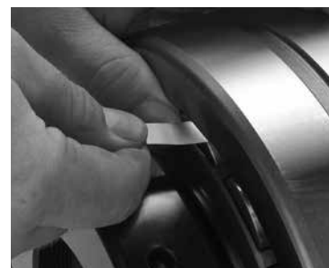
Fig. 95. Measure RIC before installation.
