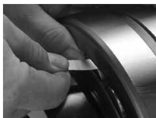
Fig. 14. Measure RIC before installation.
