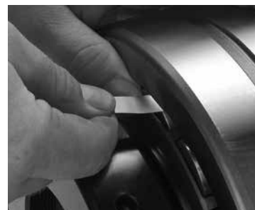
Fig. 18. Measure RIC before installation.
