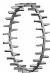
Fig. 5. EM/YM One-piece, machined-brass, roller-riding, finger-type cage.
