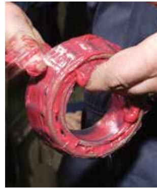
Fig. 58. Grease can easily be packed by hand.
