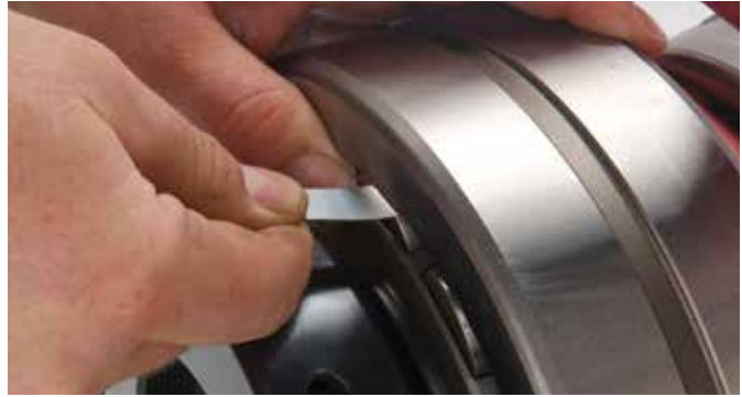
Fig. 30. Measure of RIC before installation.
