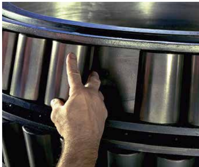
Fig. 20. Bearings must be inspected before returning to service.
