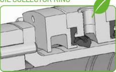
Do you prefer a clean engine room if lip seal wear occurs? Equip the Supreme® forward seal with an oil collector ring and prevent oil droplets from entering the engine room.
