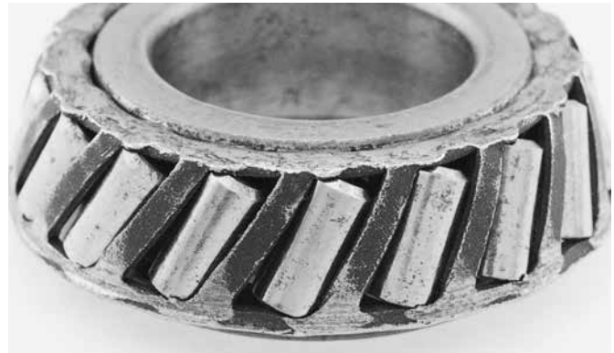
Binding and skewing of these tapered rollers was due to compression of cage ring during installation or interference during service.
