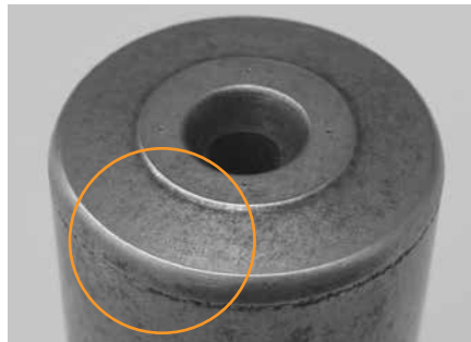
The roller end wear on this spherical bearing also was caused by fine particle contamination.
