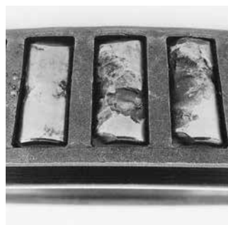
A heavily overloaded tapered roller bearing resulted in premature, severe fatigue spalling on the rollers. The load was so heavy that large pieces of metal broke off the rollers.
