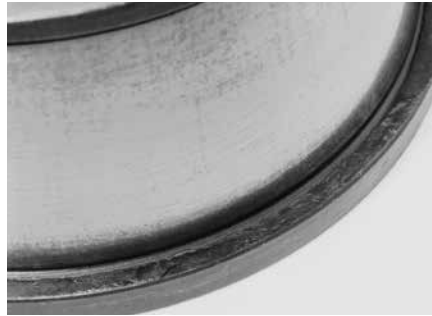
Rib and roller end heat damage.
