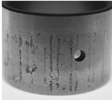
This cylindrical bearing inner ring has etching and corrosion.
