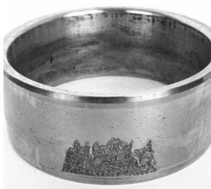
Heavy loads causing shaft deflection can lead to GSC spalling in this cylindrical roller bearing inner ring.
