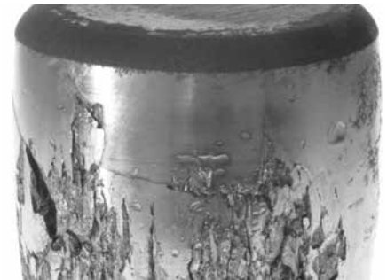
Heavy spalling and fracturing from high loads on this spherical roller bearing.
