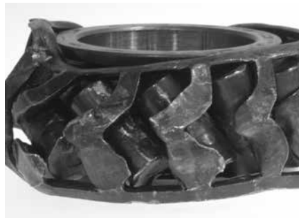
Cage damage from bearing lockup.
