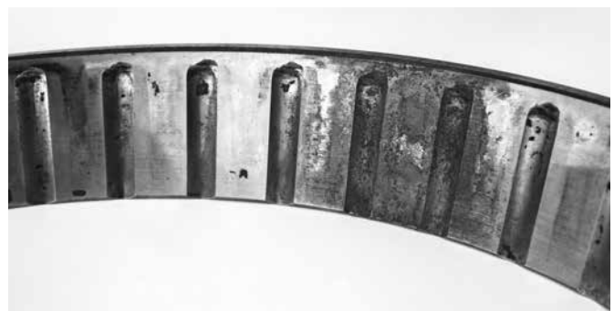
Heavy false brinell on outer race.
