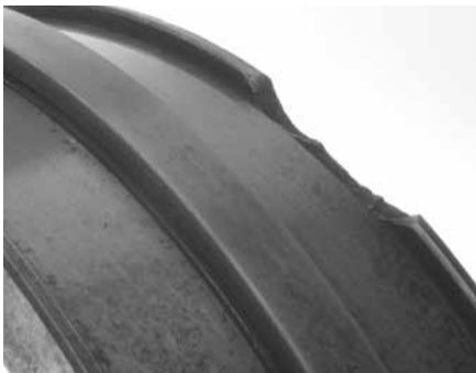
This spherical roller bearing inner race depicts a fractured small rib caused by the use of improper installation tools.
