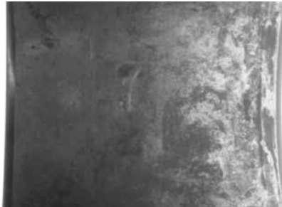
Classic fretting corrosion from poor fitting practice is depicted here. Relative movement under load between the bearing and its seat caused this worn and corroded condition.
