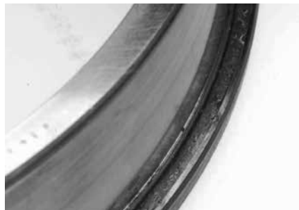
Level 2 – Advanced rib scoring is due to inadequate lubricant film.
