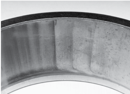
Scalloping marks in the outer ring are common with excessive endplay. This occurs when unloaded rollers enter the small load zone and are suddenly exposed to heavy loads.
