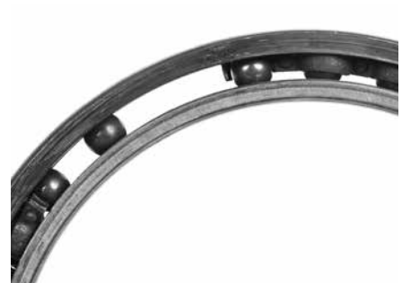
Cage damage from bearing lockup.
