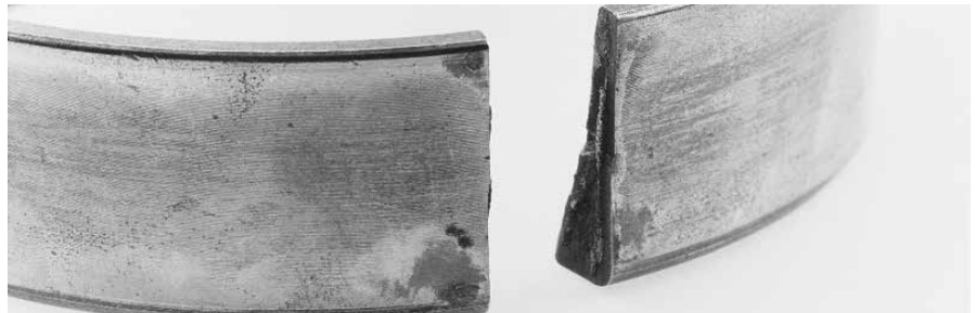
Cracked outer ring in a wheel hub. The outer ring turns and wears the outer ring seat so the fit becomes more loose. Then the outer ring starts to stretch or roll out. Wear and stretching continues to the point where the metal reaches its breaking point and the outer ring cracks open.
