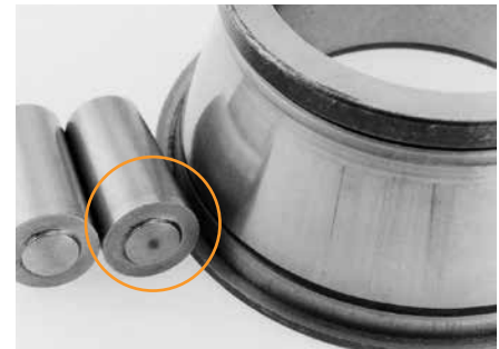
Fine particle contamination caused abrasive wear on this tapered roller bearing.
