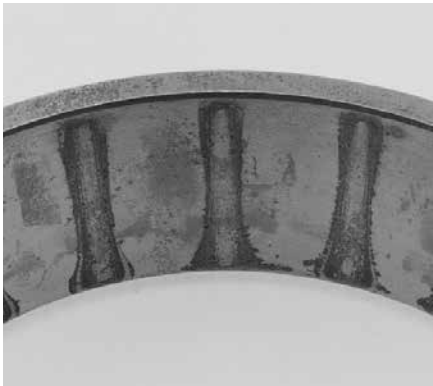
This outer ring has heavy corrosion on the race. This type of corrosion may only be a surface stain without pitting. If the staining can be cleaned with a fine emery cloth or crocus cloth, the bearing may be reused. If there are pits that cannot be cleaned with light polishing, the bearing should either be discarded or, if practical, refurbished.
