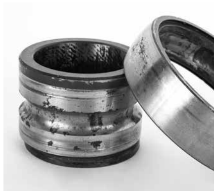
Advanced corrosion and etching.
