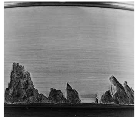
Geometric Stress Concentration (GSC) spalling.
