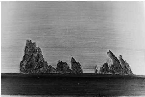
Misalignment, deflections or heavy loading on this tapered roller bearing caused GSC spalling.
