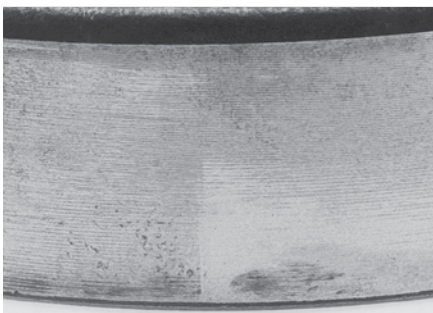
The marks visible on the outside diameter of this outer ring are caused by a high spot on the housing. The outer ring race was found spalled at the location that corresponds to the outer ring mark from heavy contact with the housing high spot.
