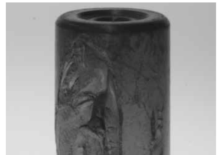
Overloading on this cylindrical roller bearing caused roller surfaces to fracture.
