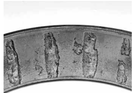
Advanced spalling initiated at water etch marks on the outer ring race makes this bearing unsuitable for further service.
